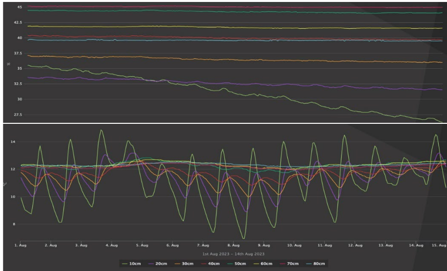
Figure 25. Soil moisture content (top) and soil temperature (bottom) at depths of 10 cm to 80cm at 10 cm intervals as displayed by the green brain platform online.
