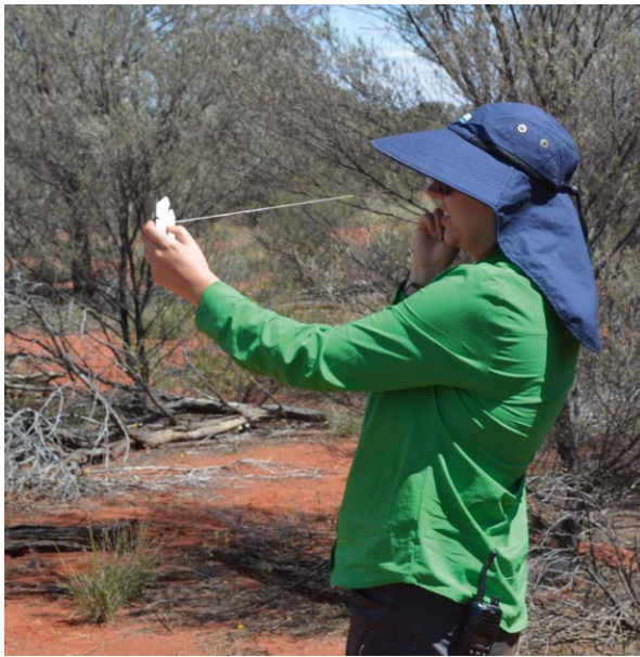
Researcher Isabelle Wagelmans uses a basal wedge to collect measurements that will help estimate Mulga cover
